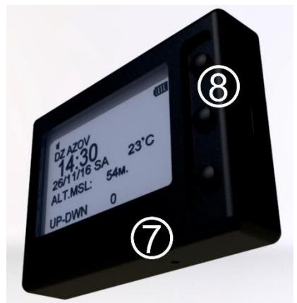
Use buttons "**Up**" and "**Down**" to move through the menu. "**Select**" is used to choose.
