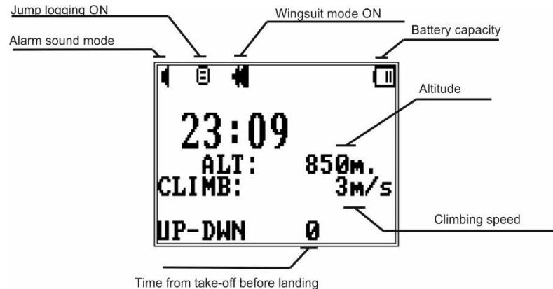
The altimeter automatically switches to the altitude gain mode. When the altitude is 300 meters, the device beeps and the indicator flashes (5) which means switching to the altitude gain mode. In case of very slow dialing, the device may not automatically switch to the dialing mode, in this case it can be transferred to the “In flight” mode in the manual mode, from the “Setup” menu. If the jump did not take place, the altimeter independently switches to the “On the ground” mode.
